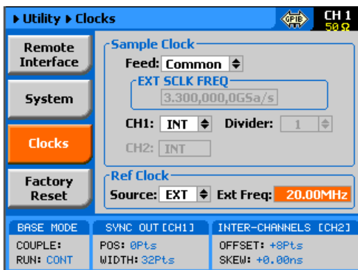
Figure 3-16, Using an External Clock Reference Example
