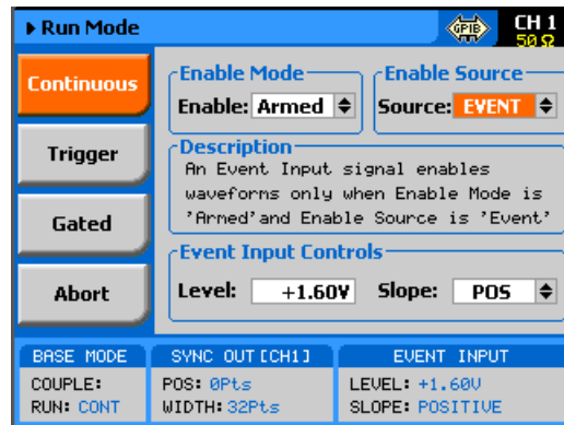
Figure 3-10, Typical Continuous Run Mode Display with the Abort Soft Key
