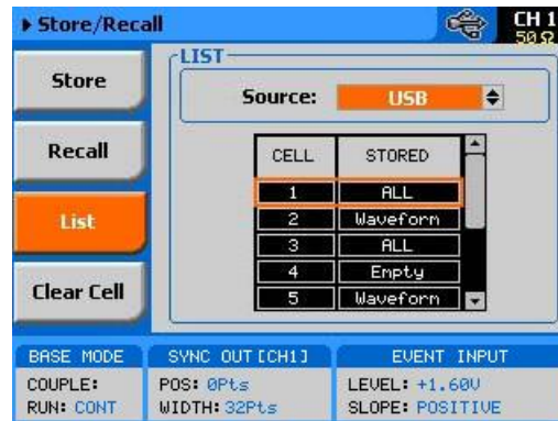
Figure 3-81, Stored Memory Cells Listed
