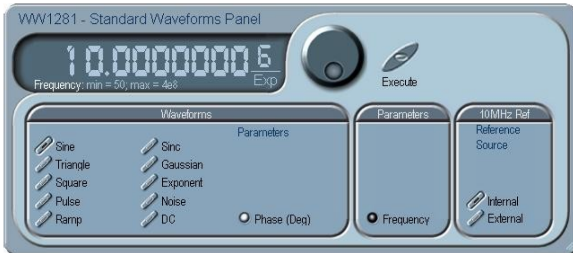
Figure 1-11, ArbConnection Example - Typical Standard Waveforms Panel
