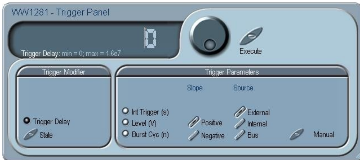
Figure 4-9, the Trigger Panel
