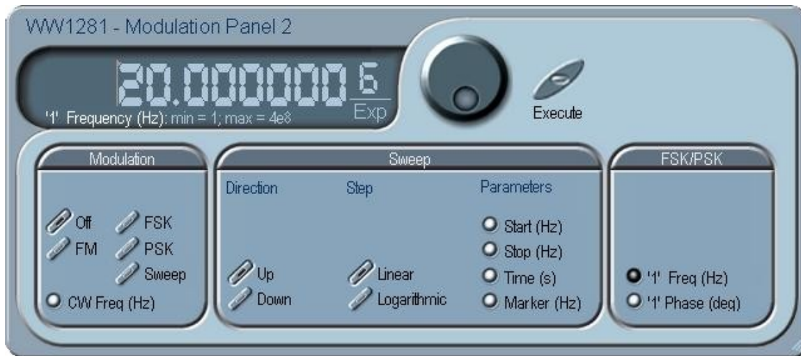
Figure 4-11, the Modulation Panel 2
