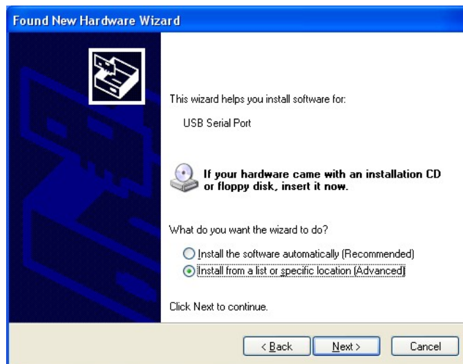
Figure 2-11, Found New USB Serial Port
