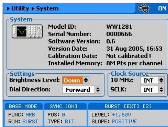
Figure 03-13, Modifying the SCLK and 10MHz Clock Source
