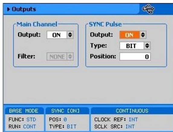
Figure 03-12, SYNC and Filter Parameters
