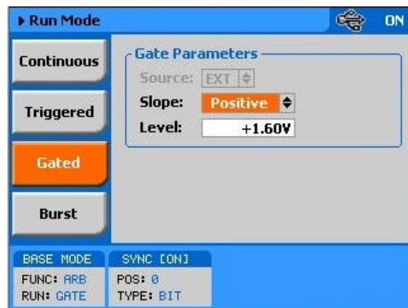
Figure 03-10, Gated Mode Parameters
