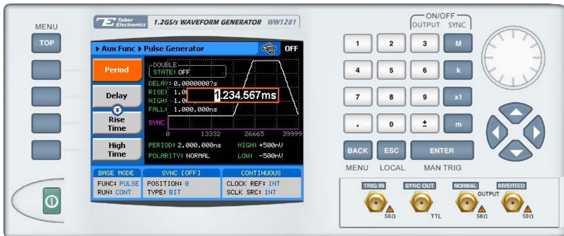
Figure B-3, Programming the Pulse Period Parameter
