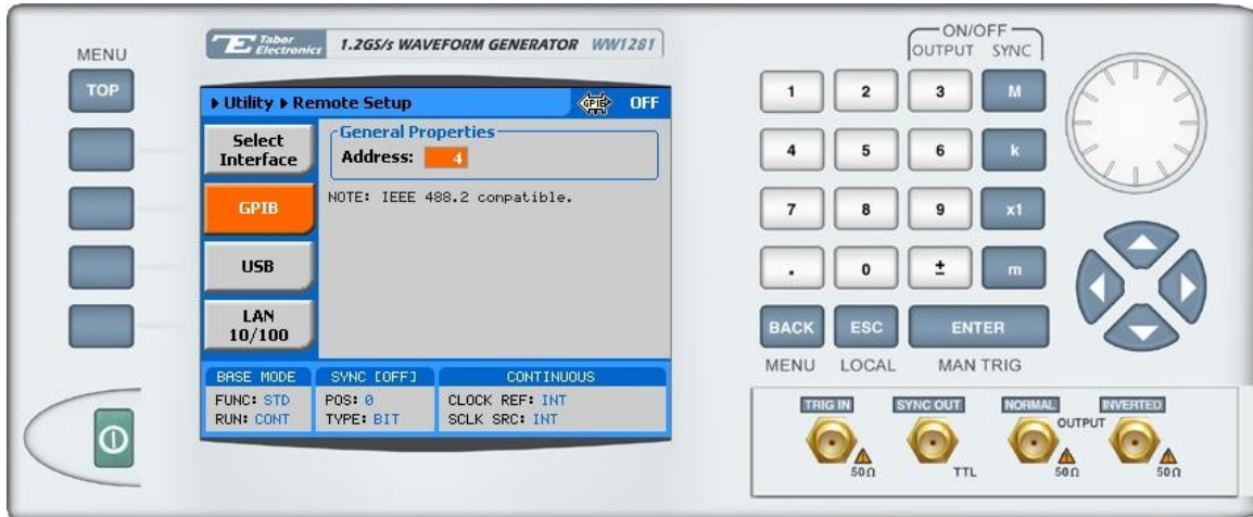
Figure 2-2, GPIB Configuration Screen
