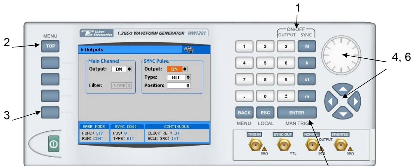
Figure 03-3, Enabling and Disabling the Outputs
