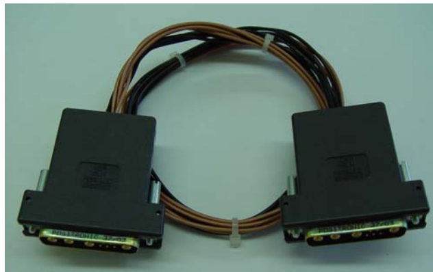
Figure 3-39, the 1281A Synchronization Cable
