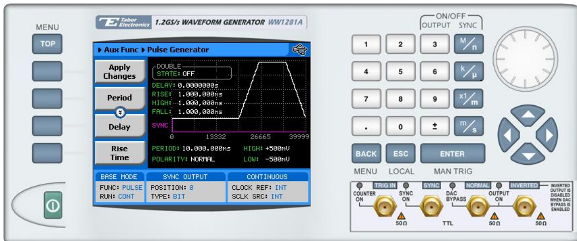
Figure 1-25, 1281A Digital Pulse Generator Menu Example
