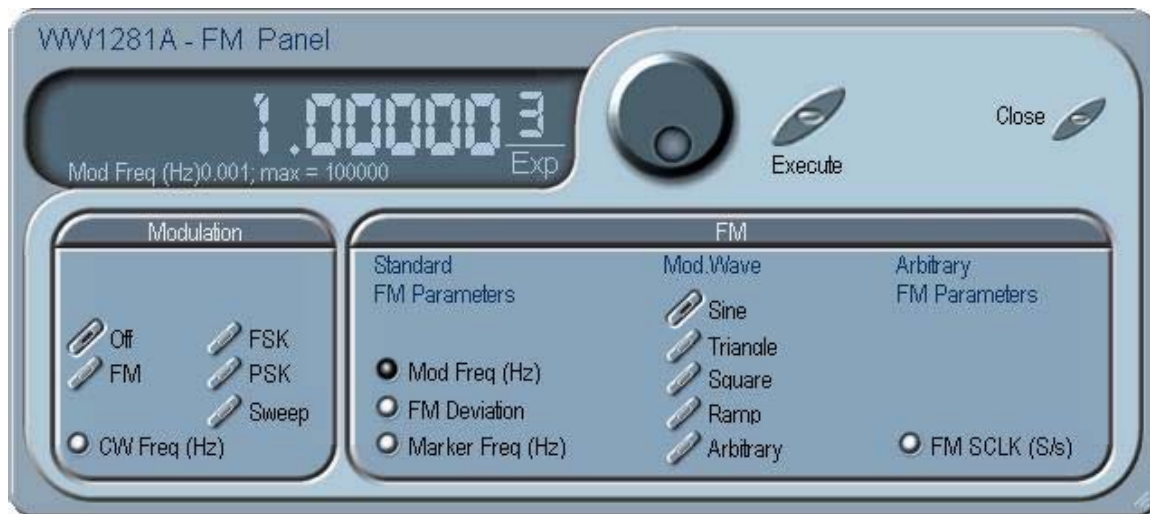
Figure 1-23, ArbConnection Example – FM Panel
