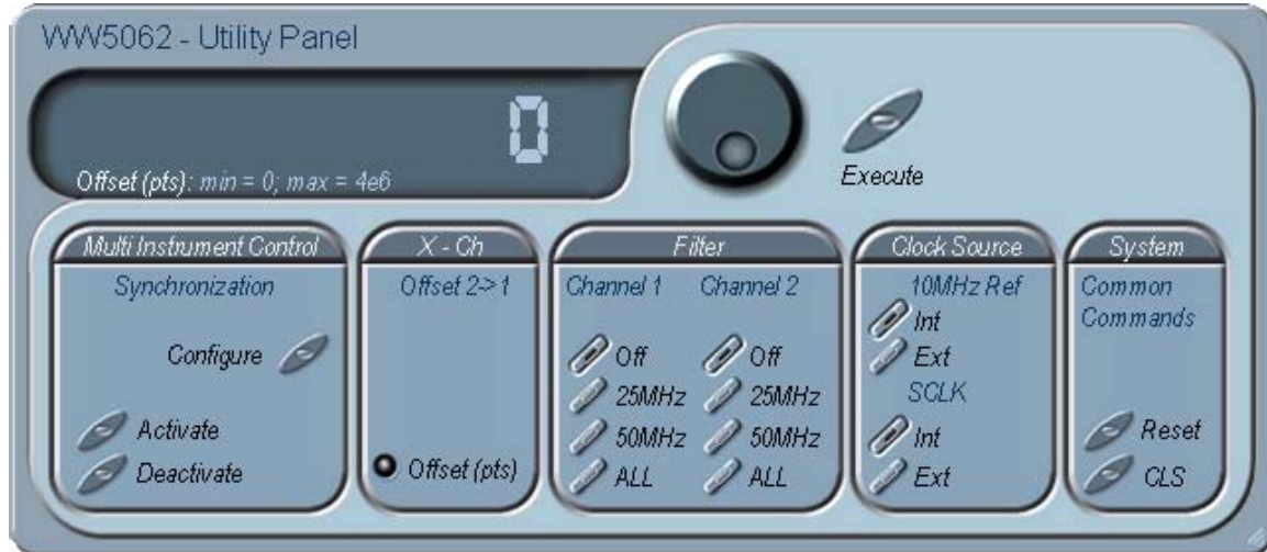
Figure 4-12, The Utility Panel
