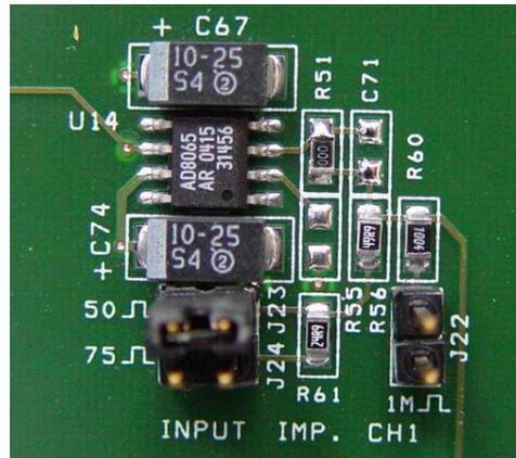
Figure 2-1, Field Modification of Channel 1 Input Impedance
