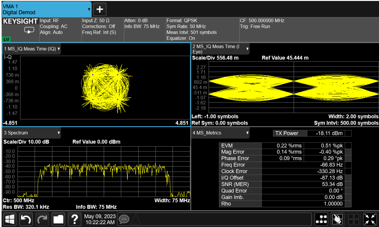
Figure 13-9 500MHz QPSK Signal Analysed with a VSA
