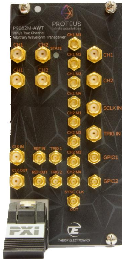
Figure 10.14 Proteus P9484M-AWT Front Panel
