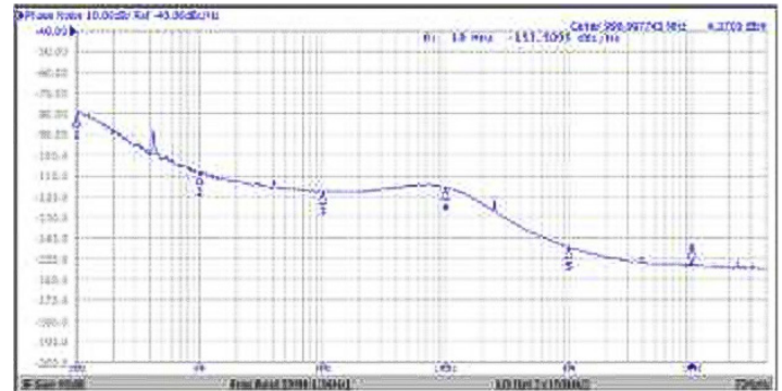
Figure 5. Phase Noise Plot of 1 GHz Signal
