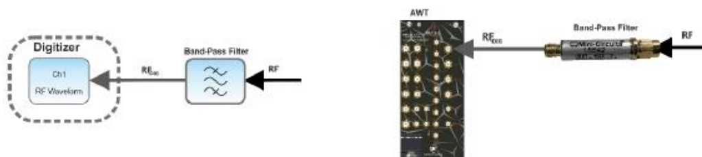
Figure 2.4 Capture of RF Signals Using a Digitizer
