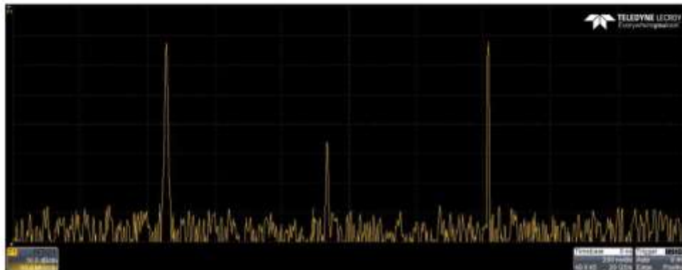
Using the internal NCO (Numerically controlled Oscillator) to Amplitude Modulate 125Mz waveform file – Frequency Domain
