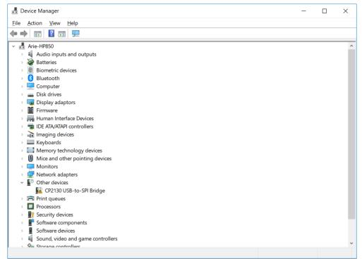
8. In the navigation tree, expand Other devices and double click on CP2130 USB-to-SPI Bridge.
