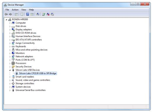
13. In the CP2130 USB-to-SPI Bridge Properties window the device status should indicate the device is working properly.
