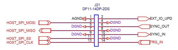
**Figure 5.2 SPI Connector Pad Description**
