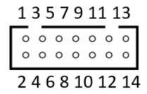
Figure 5.1 SPI Connector Pin Numbering
