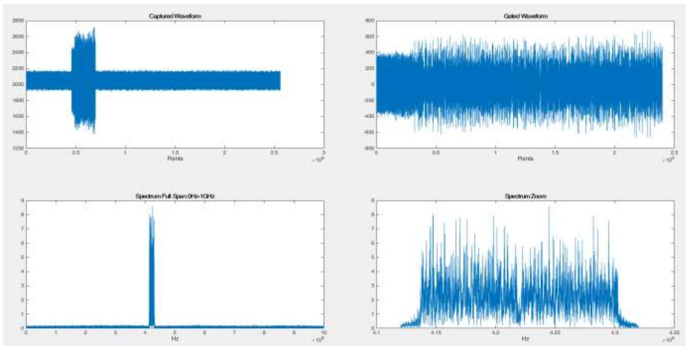
The above plots also have random noise added and I used a filter to eliminate any spurious signals. More measurements are possible using the rich signal processing toolset within MATLAB including modulation quality, adjacent channel power and CCDF.
