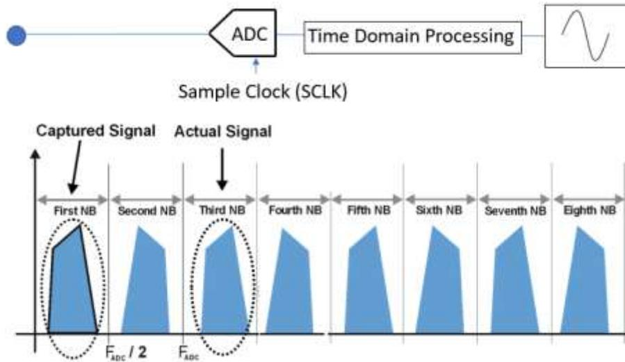
Referring to the above figure – when we sample a 2.4GHz signal with a 2GS/s clock ( $F_{ADC}$  or SCLK) we will see an undersampled image of the signal in the first Nyquist Zone or at 400MHz (2.4GHz-2GS/s).
